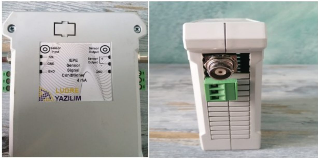
Figure 2. IEPE Setup Signal Conditioner with IEPE Acoustic Microphone
