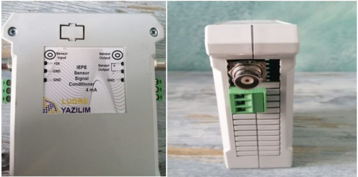
Figure 3. IEPE Setup w/Signal Conditioner
