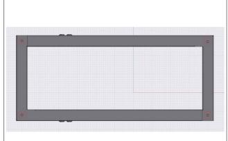
Mounting to the machines is possible with the bolt and nut assembly in the areas indicated in the adjacent image. The points to be taken into consideration during this installation are as follows: The electronic parts should not be contacted while assembling the product. In addition, if the product is not installed properly, vibrations that may occur will cause errors during measurement and control.
